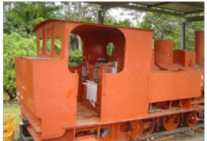
Boiler fittings mounted on the firebox. Most of these items had been stripped from the loco before we received it. With no old photos of these items, we have had to exercise our originality.
